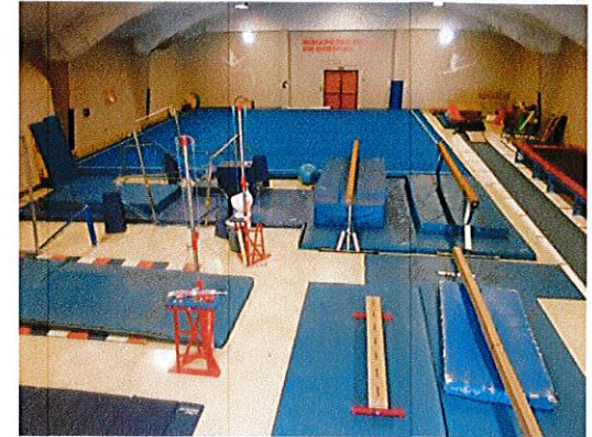
Photo 6: Create wheelchair viewing positions on the gymnastics floor (because there is not an accessible route to the viewing loft).
