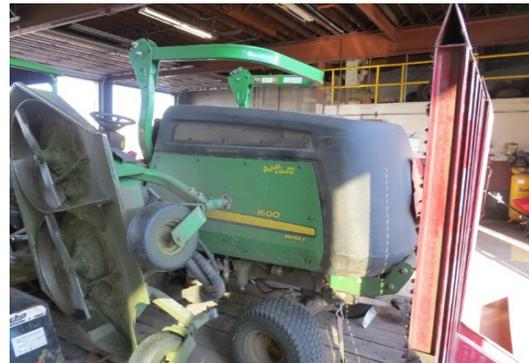
Fun Fact: This unit has 3 different mowing decks (2 side decks and a front deck) that can be operated independently of each other for increased efficiency.
