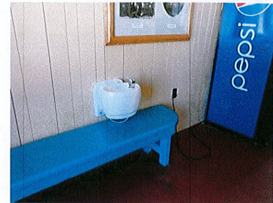
Photo 3: Relocate the bench; it currently obstructs access to the drinking fountain.
