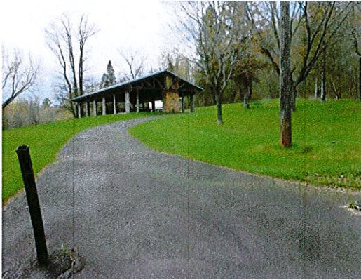
Photo 1: The slope of the route from parking to the picnic pavilion is currently 9.5%.
