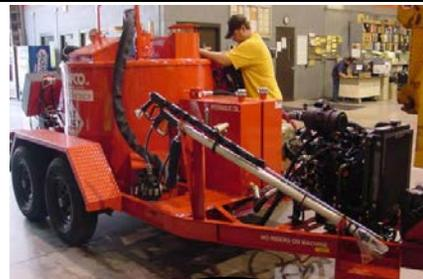
Fun Fact: This is used to melt and apply about 80,000 lbs of sealant to fill a crack that is 2" wide by 2" deep and 5 miles long (cool hey!). Not so fast, remember we have 450 miles of streets that are on average 32' wide (that's nothing to crack up about!).
